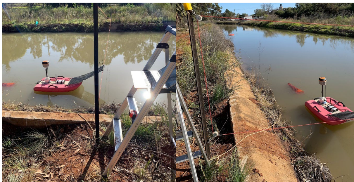
Figure 7: Cableway Design at each Measurement Site for ADCP Discharge Measurements.
