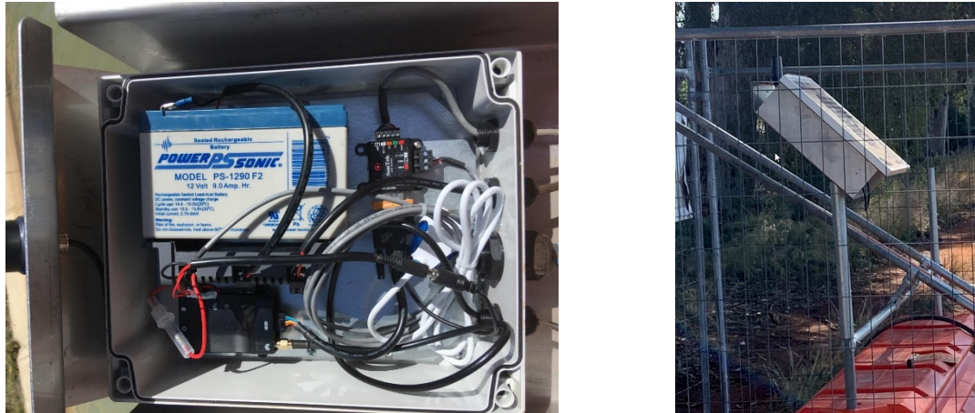
Figure 6: Junction Box for Housing Electronics
